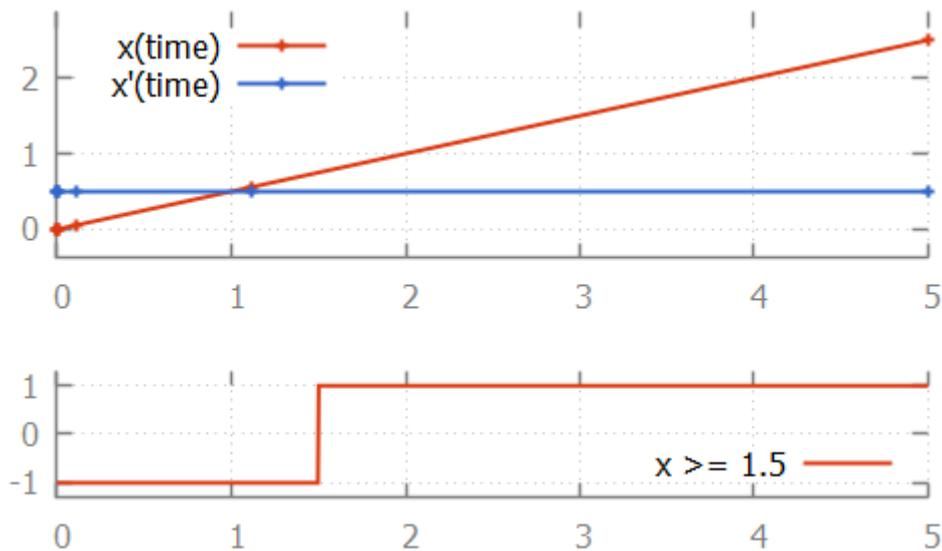
we see that at time 1.1111, the value of the guard is -1 (false). At time 5.0 it is +1 (true). That is, the guard changed value between two time points calculated by the integrator. If this is the case, the ODE solver tries to calculate the exact time point at which the guard changes its value. That is, it calculates the exact time point at which the guard function crosses the time axis, and thus has a root.
