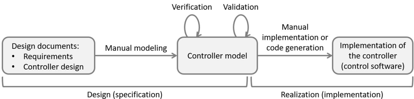
At the center is a controller model, a model of a controller that unambiguously specifies how the controller works. It precisely specifies how the state of the controller changes when a sensor signal changes, and under what conditions and in which states an actuator may be turned on or off. Ideally, the model has a mathematical foundation. It may for instance be modeled as one or more state machines.
