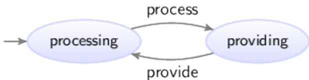
The states are labeled with the names of the current locations of automaton `machine1`. Since automaton `machine2` has only a single location, its current location does not change, and it is therefore not included in the state names.
