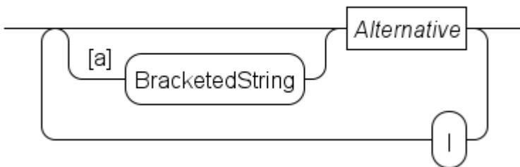
The **BracketedString** like **[a]** can be used to denote specific points in the diagram allowing you to refer to such points from the explanatory text.
