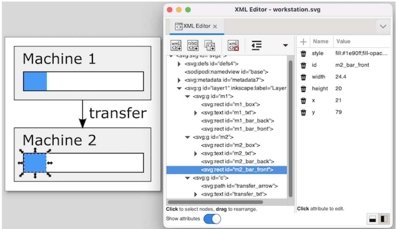
In the image, two machines are clearly visible. Each machine has a bar that shows the progress of the machine. Looking at the *XML Editor* window, we can see the bar has a background (box), and a foreground (front) rectangle. The **width** and **fill** color of the latter will be updated to reflect the machine's status.
