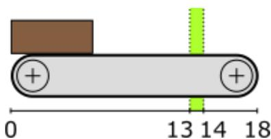
The product starts at the left side, at position **0**. There is a sensor that can detect the product between positions **13** and **14**. The product exits the conveyor at position **18**. The following CIF specification models the conveyor, product, and sensor:
