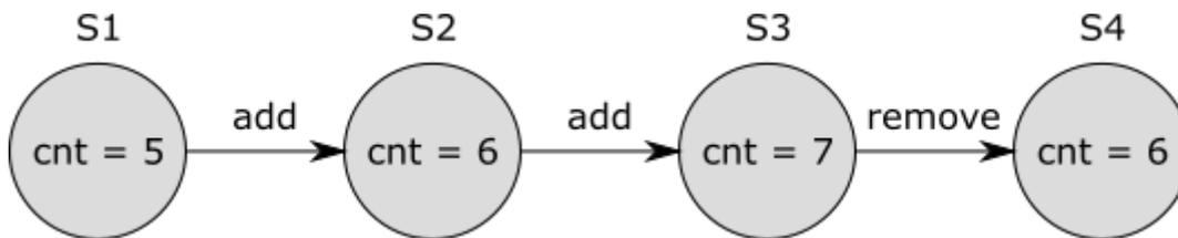
In the initial state (S1), variable **cnt** has value 5. An item is then added (transition for the event **add**), resulting in a new state (S2), where **cnt** has value 6. After that, another item is added, leading to state S3, where **cnt** has value 7. Finally, an item is removed by means of a transition for event **remove**, leading to state S4, where **cnt** has value 6 again.
