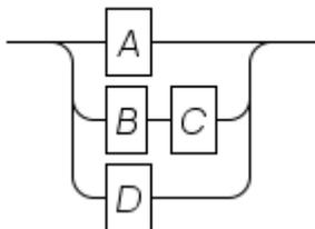
Note that as sequence has higher priority than choice, the **B** and **C** sequence forms one alternative. You can use parentheses to break the priority chain, e.g.:
