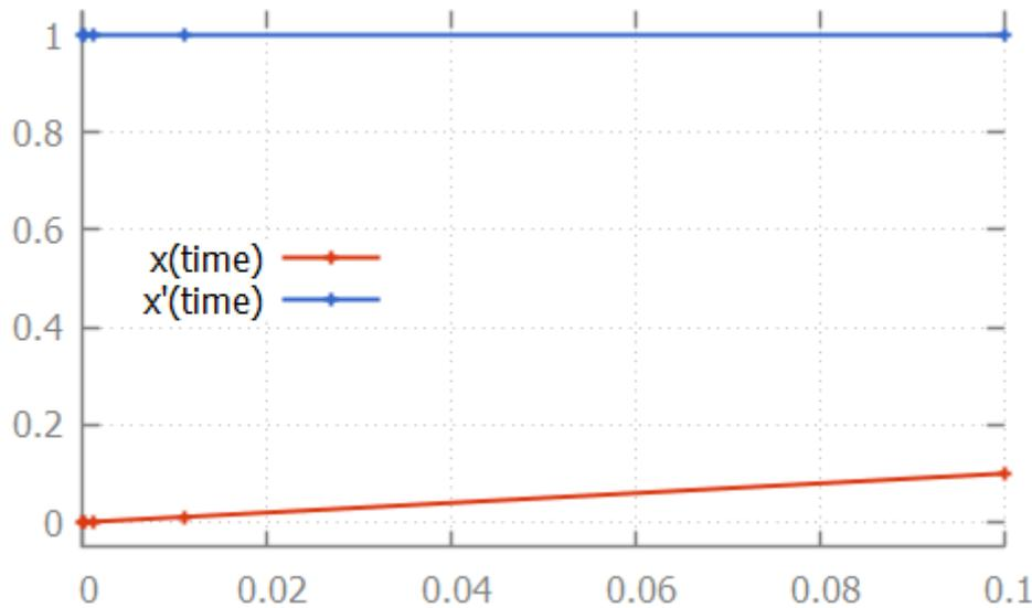
Here, the numerical integrator start with the initial value of continuous variable  $x$ , which is  $0.0$ . For the initial value of variable  $time$ , which is also  $0.0$ , it computes  $x'$ , which is  $1.0$ . It then slightly increases the value of variable  $time$  to say  $1e-6$ . Assuming a linear continuous variable  $x$ , the value of variable  $x$  at that time is  $1e-6$  as well.
