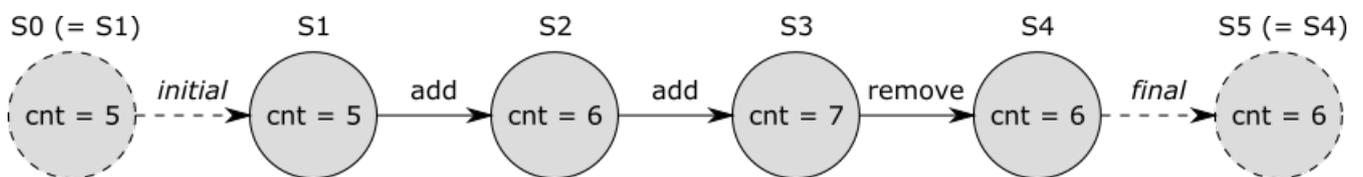
A transition with the *initial* label is added before the initial state, and a transition with the *final* label is added after the final state. This ensures that all states have an incoming and outgoing transition. These two added transitions are *virtual*, they don't actually exist. They are added only for the benefit of print output. That is, they don't affect the behavior of the model, and are thus not part of the 'real' trace.
