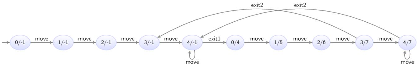
The states are labeled with the values of the **pos** variables of the automata for the first and second conveyors.
