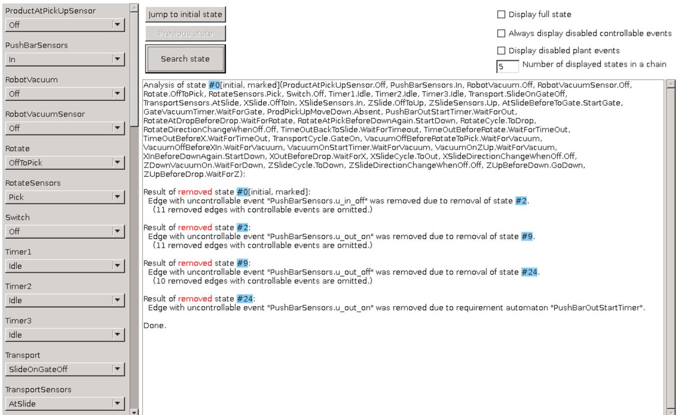
This is an example from a bigger system, where the supervisor is empty. The analysis of the initial state reveals that it was removed due to a removal of a chain of other states. State #24 was removed due to a requirement (reading from bottom to top), which caused the chain of states #9, #2, and eventually #0 to be removed.
