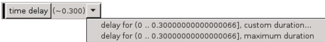
At most  $0.300000000000000066$  units of time can pass ( $0.300$  in short form). The first option is to choose a custom duration. The second option is to choose that maximum duration, similar to clicking the **[ time delay ]** button. The following image shows the dialog that is presented to the user to enter the custom duration:
